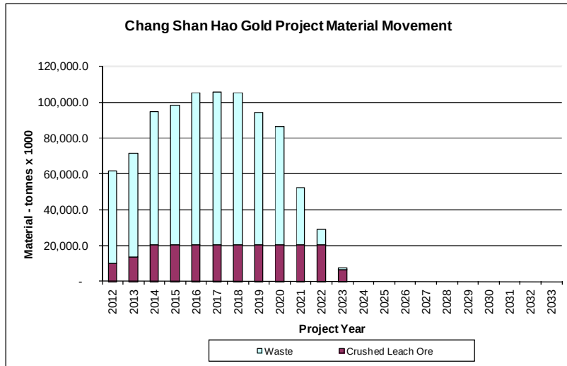
Figure 16-4 Material Movement Schedule
